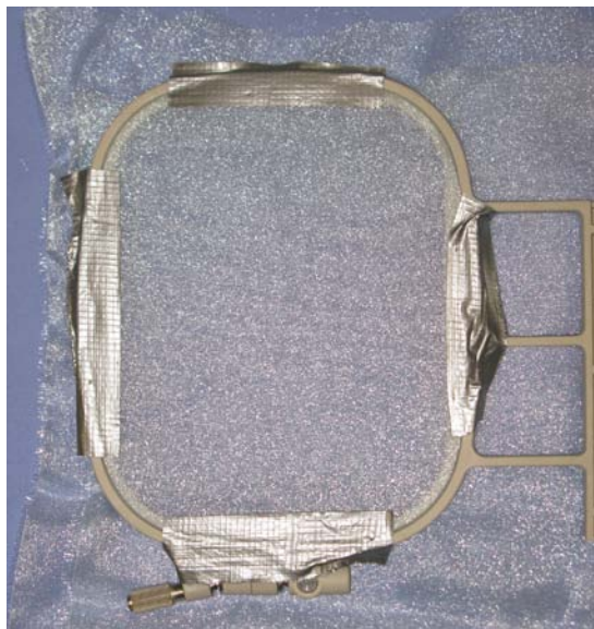
Figure 4. Duct tape is another technique for slip prevention. Strips are cut in half lengthwise and wrapped around the edge of the hoop from the back.
