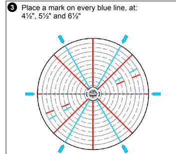
Place the Template Marker on each set of points with the arrow facing OUTWARDS and mark points. When embroidering, ensure each design is hooped square with the arrow upright.
