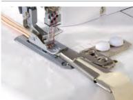
You can easily make a belt loop simply by setting and feeding your fabric into the belt loop folder attachment.
