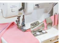
The Knit Binders will turn fabric strips into binding and attach to your project edge all in one step to give you a professional finish.
