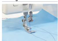
The Curve Foot is suitable when stitching a curve because its length is short and sole is flat.
