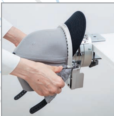
Sliding and ratchet frame fixing
