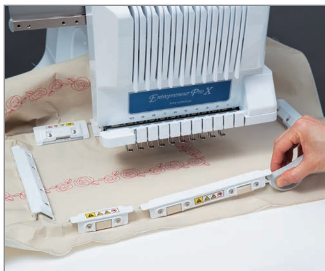
Included Leverage magnet lifter, easy to remove the magnetic pieces
