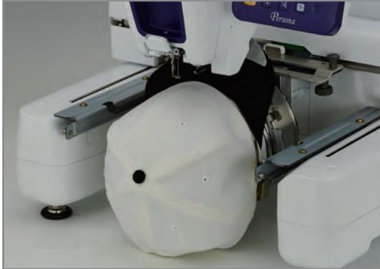
Set completed cap directly onto the machine
