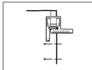
When using a marking pin, always remove it before it can pass under this foot.
