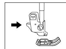
2. Loosen the screw of the presser foot holder to remove the presser foot holder.
