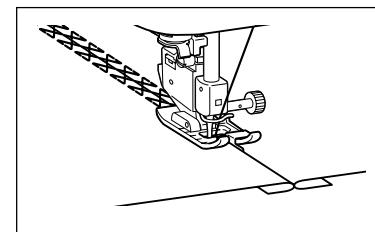
After sewing two pieces of fabrics together, this foot can be used to sew decorative stitches over the seam (ditch). Sew two pieces of fabric together using a straight stitch. Press the seam open. With right side of fabric facing up, place the guide of the foot in the seam (ditch). Select a decorative stitch and sew.
