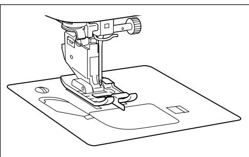
Change the presser foot to the edge joining foot.
