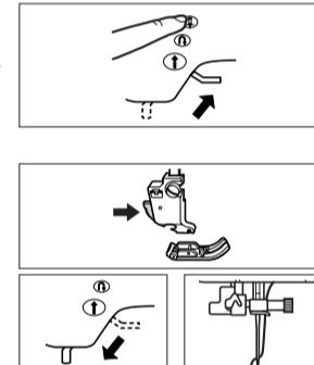
**Caution:** The needle threader cannot be used after attaching the side cutter. Using the needle threader may result in damage to the machine while attaching the side cutter. When rethreading, be sure to thread the needle after removing the side cutter.
