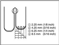
It is convenient to use the markings on the presser foot as a guide when sewing narrow seam allowances, decorative stitches, etc.
