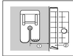
When sewing a margin wider than 8.5 mm ①, you may find it helpful to attach a piece of tape to the needle plate ② to help guide the fabric.
