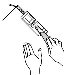
5. After sewing 2 to 3 cm of the fabric, release the thread and guide the fabric from the front of the presser foot with your left hand. Keep a uniform amount of fabric wrapped around the presser foot curl until the seam is completed.
