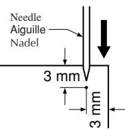
1. Position the fabric (reverse side facing up) under the presser foot. Lower the needle 3 mm from the edges of the fabric, lower the presser foot, then sew 2 or 3 stitches.
