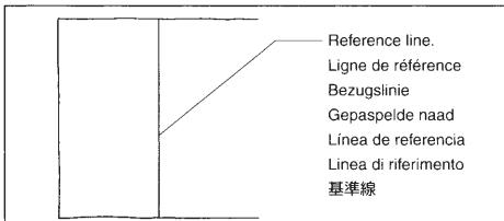
Position the fabric so that the reference line is on the side of the space in the middle of the presser foot.
