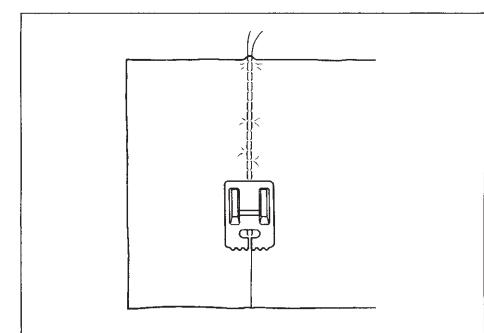
To create a second pin tuck perfectly spaced from the first, simply raise the presser foot and position the first pin tuck under one of the grooves in the foot. The foot will use the first pin tuck to guide its sewing the second pin tuck. The distance between each set of pin tucks depends upon which groove the guiding pin tuck is placed.
