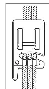
Draw cording under foot and extend the cord 4-5mm behind foot. When using 2 or 3 cords, be careful to make sure that cords are not trampled under the front of foot.
