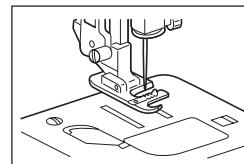
Remove presser foot and attach snap-on cording foot.
