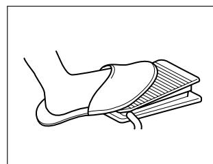
Using your foot controller will help you to have both hands free for easier fabric handling. (Some machine models do not include the foot controller, check your instruction manual for the part number and ordering instructions.)
