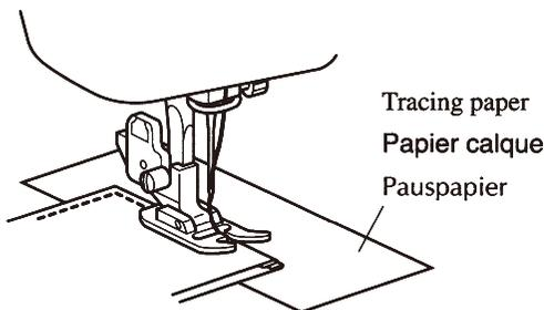
If feet at the needle plate is hindered by the fabric's surface, place thin paper such as tracing paper beneath the cloth and resume sewing.
