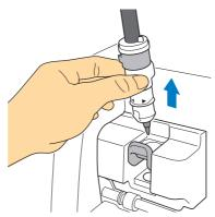
Push down on the release lever on the calligraphy stand, place the pen holder (with a pen installed) in the calligraphy stand so that ◀ on the holder aligns with ▷ on the front of the stand, and then return the release lever to its original position.
