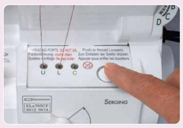
ExtraordinAir™ with Tubular Loopers allows you to thread in any order and avoid tangles and knots as threads are not exposed.
