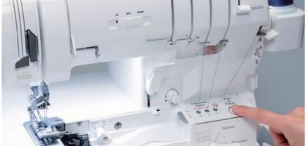
Simply push the button and air blows the thread through the tubular loopers.
