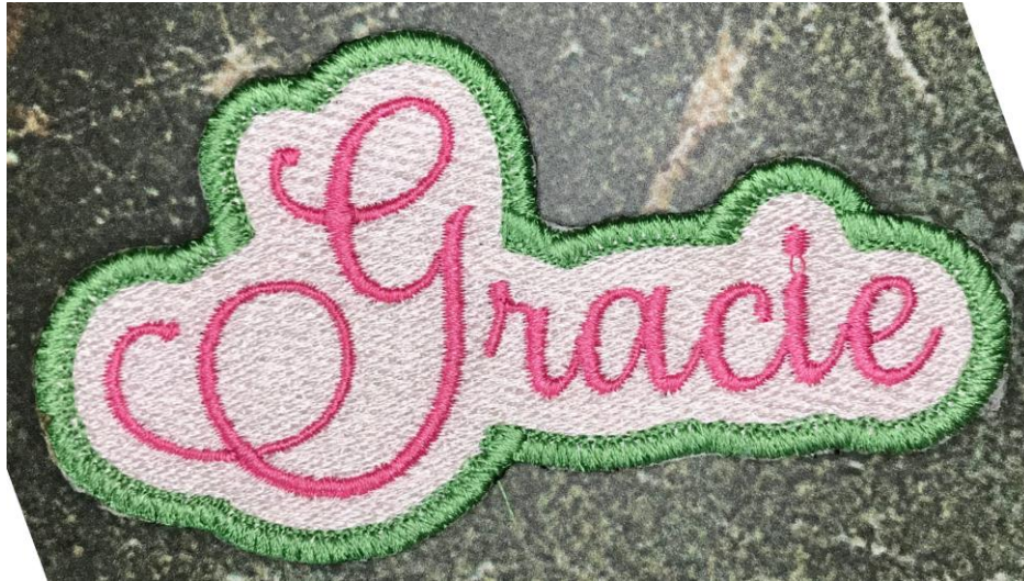
Testing a complex shape using no fabric. Note edge needs final treatment.
