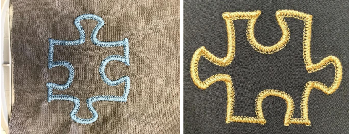
Left: The trouble with not fusing your twill. Right: Fused sample. Shape impossible for a real overlock machine.
